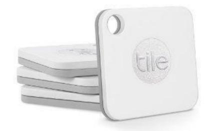
Small GPS enabled devices that can be attached to keys, wallets, electronics and anything that you want to track. Items can then be located using a app on the cell phone.
